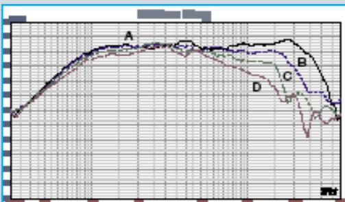
FIGURE 3: 28-537SH horizontal on- and off-axis frequency response (A = 0°; B = 15°; C = 30°; D = 45°).
