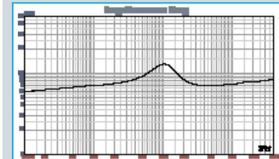
**FIGURE 8:** Tang Band 28-1582S free-air impedance plot.
